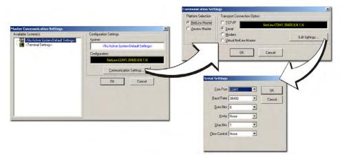
FIG. 23 Assigning Communication Settings and Baud Rates
